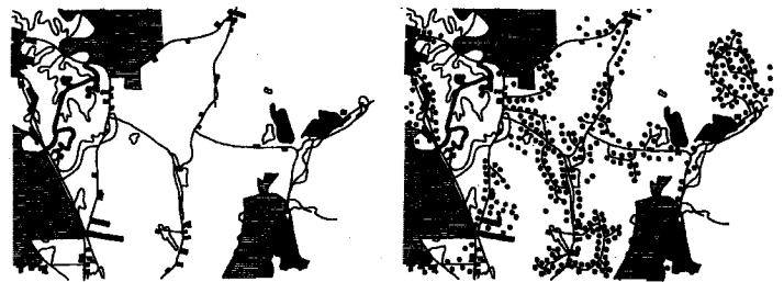
Figure 2 A matching pair of graphics, taken from an actual "build-out map," showing existing conditions (mostly undeveloped land) contrasted with the potential development pattern of "checkerboard suburbia" created through conventional zoning and subdivision regulations.
